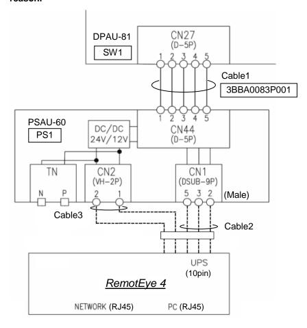
Figure 4-24 Connection between Display Control PCB (SW1) and RemotEye® Module
