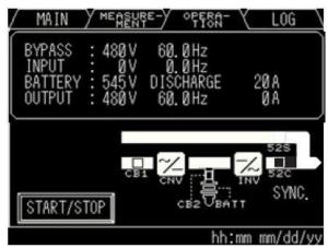
Figure 5-27 Open Battery Breaker
