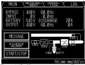
Figure 4-15 Measurement screen (Battery Operation)
