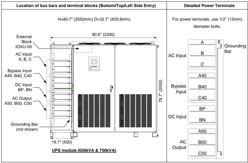
Figure 5-4 Diagram of input/output bus bars and terminal blocks (650kVA & 750kVA)
