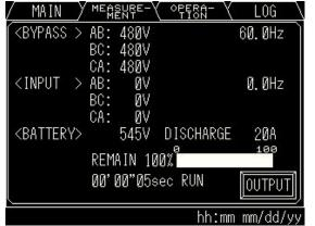
Figure 4-14 Main Screen (Battery Operation)
