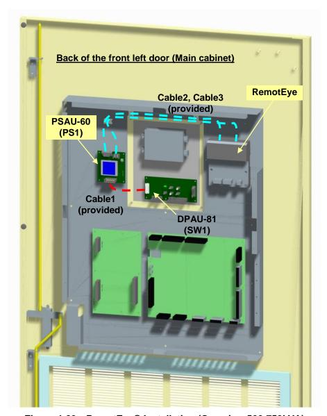
Figure 4-23 RemotEye® Installation (Overview 500-750kVA)
