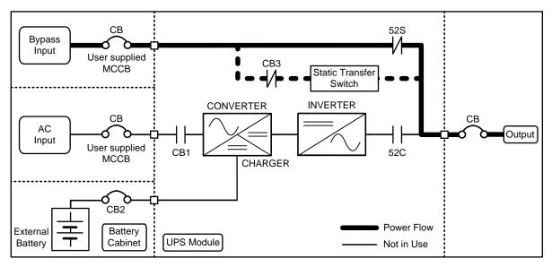
Figure 3-2 Single Line Diagram – Bypass Operation: Load fed through static bypass line.
