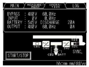
Figure 5-26 UPS Transfers to Bypass
