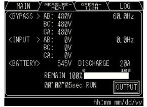
Figure 4-7 Battery Operation Values
