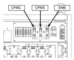
Figure 5-19 Circuit Protectors Location
