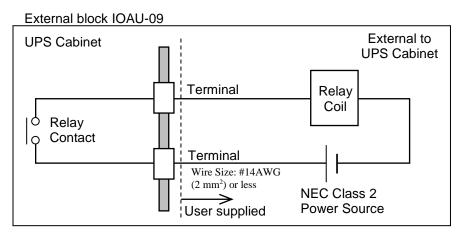
Figure 4-20 Control Wiring for Aux Output Contacts
