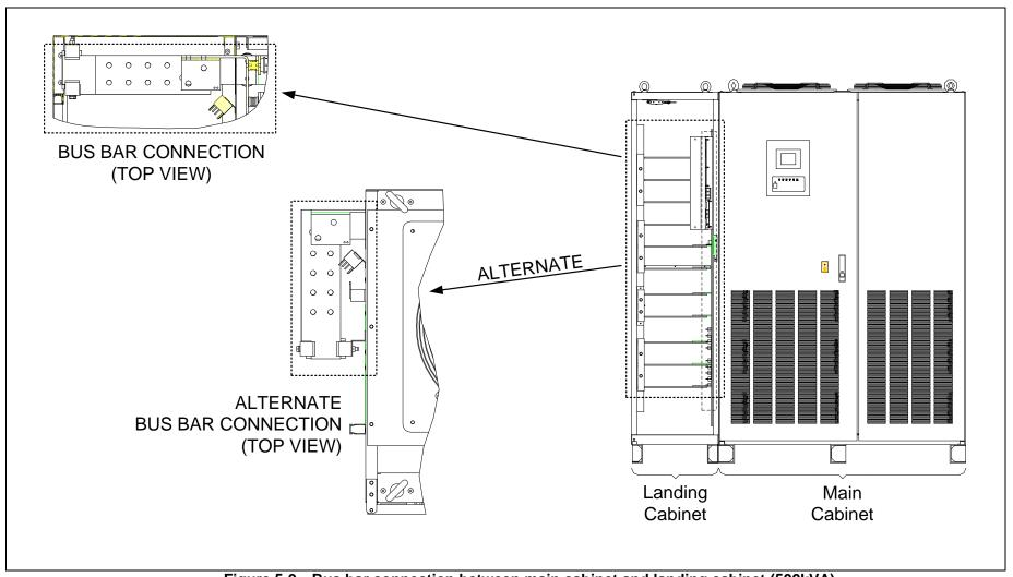
Figure 5-9 Bus bar connection between main cabinet and landing cabinet (500kVA)
