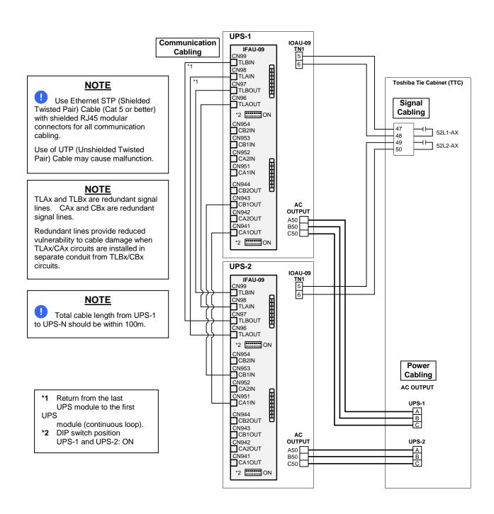
Figure 5-13 Diagram of Communication, Power & Control Wire Connections for 2 units in MMS Configuration (300-750kVA)
