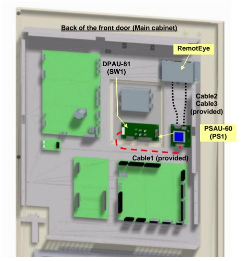
Figure 4-22 RemotEye® Installation (Overview 300kVA)
