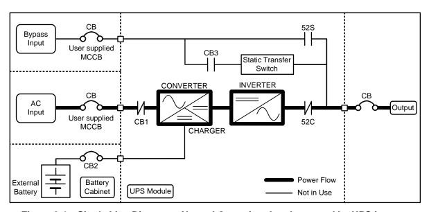
Figure 3-1 Single Line Diagram – Normal Operation: Load powered by UPS inverter
