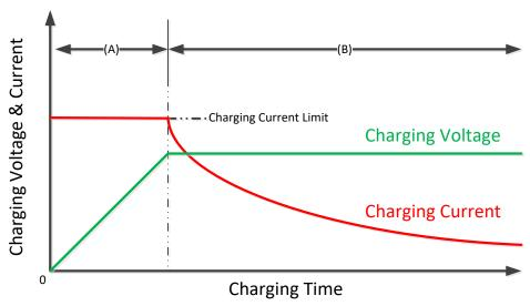
Figure 3-4 Typical Battery Charging Curve
