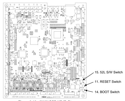
Figure 3-12 MAIN PCB UPJR-C\*
