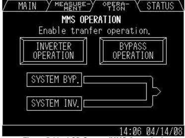
Figure 5-28 LCD Screen (MMS Operation)
