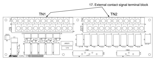
Figure 3-9 External I/F PCB IOAU-09
