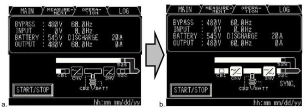
Figure 5-20 Automatic Startup of Inverter and Converter
