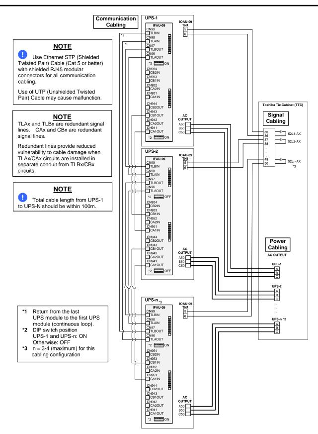
Figure 5-15 Diagram of Power Wire & Control Wire Connections for 3-4 units in MMS Config. (300-750kVA)
