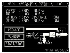
Figure 4-16 Main screen (Fault indication)
