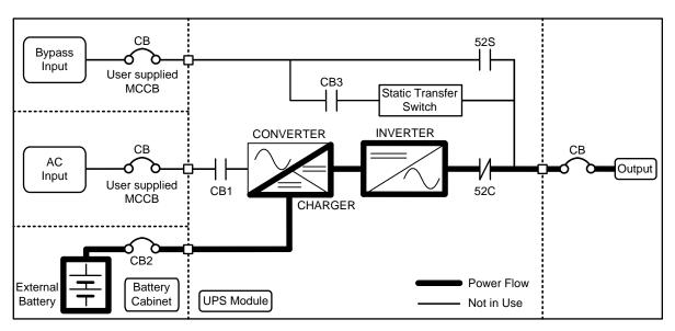
Figure 3-3 Single Line Diagram – Battery Operation
