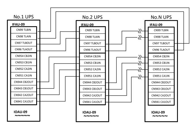
Figure 5-18 Detail of IFAU-09 Control Wire Connections for 5 to 8 units in MMS Configuration (300-750kVA)
