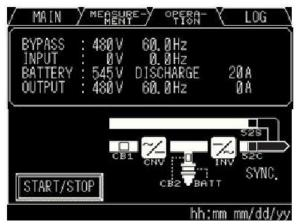
Figure 5-21 Close Battery Breaker
