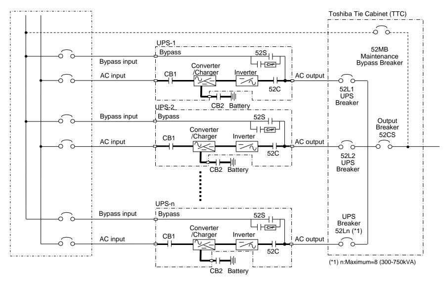
Figure 5-12 Diagram of Power Wire Connections (Parallel System Configuration)
