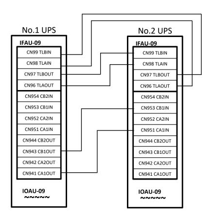
Figure 5-14 Detail of IFAU-09 Control Wire Connections for 2 units in MMS Configuration (300-750kVA)
